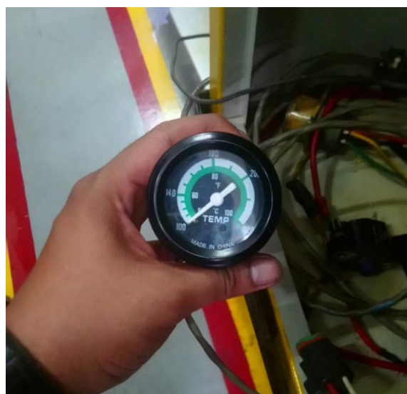
Gambar. 3. Indikator coolant water temperature
