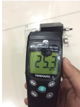
Gambar 3 Solar Power meter
