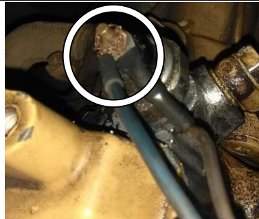
Gambar 7. Pemeriksaan Engine Oil Pressure Indicator
